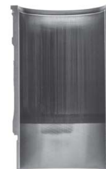
Severely Scuffed Liner
